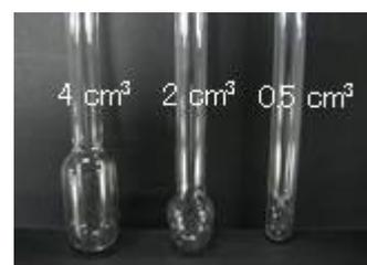
Fig. 4 Measuring cell for gas adsorption method
