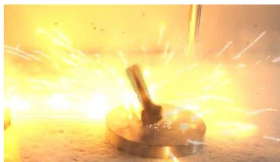
Fig.2 Impact sensitivity test
