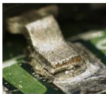
Example of peeling of solder on terminals
