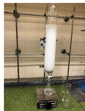
Fig. 2 Purification by column chromatography
