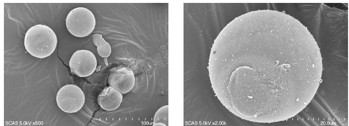
Fig.1 SEM images of Silica particles
