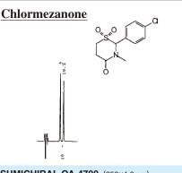
**SUMICHIRAL OA-4700** (250×4.6mm) Mobile Phase : hexane / 2-propanol / methanol / trifluoroacetic acid (80 / 15 / 5 / 0.2) :1.0mL/min :UV254nm Flow Rate
